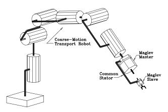
Figure 1: Proposed System Configuration
