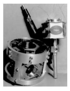
Figure 5: Micro-wrist stator and flotor
