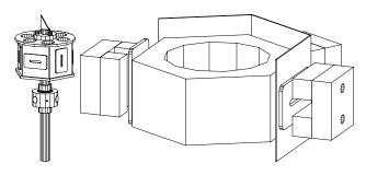
Figure 6: Flotor and Actuator Configuration
