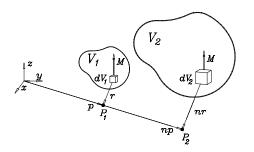
Figure 3: B-field scaling from a magnetized body
